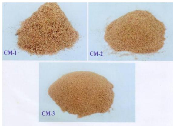
Figure (1) Three Different Mesh Sizes of Coconut Mesocarp Samples
