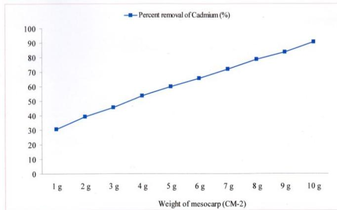
Figure 3. The Plot of Percent Removal of Cadmium by using Various Weights of Mesocarp (CM-2) Sample
