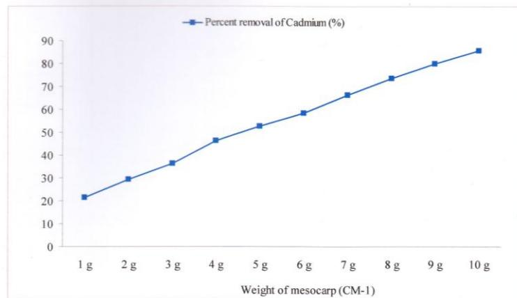
Figure 2. The Plot of Percent Removal of Cadmium by using Various Weights of Mesocarp (CM-1) Sample
