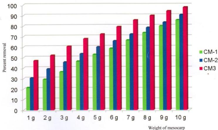
Figure 5. The Histogram of Percent Removal of Cadmium by Using Various Weights of Three Different Sizes of Mesocarp Samples
